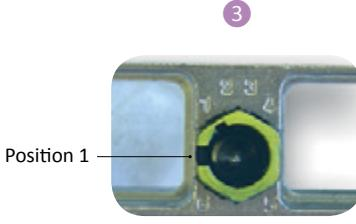
**Key polarizing are always mounted on Plugs.**
