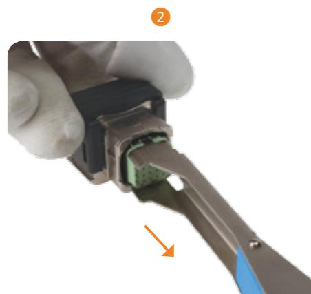
① Place the tool at the rear of the shell. Push the tool gently along the side of the module until it meets a clear resistance, at this point the locking system have been released.
