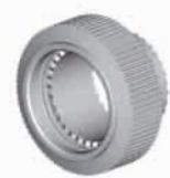
**Type 1:** Adaptor for use with a standard 38999 Series III/EN3645 backshell. Caution is necessary in the choice of the standard backshell: it must allow enough room to accommodate the push back of the cable during the connector mating.
