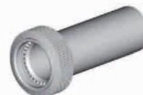
**Type 4:** Backshell derived from Type 3 without the cable gland. Suitable to adapt specific male threaded adaptors (not supplied) for ANAMET or PMA tubes for example. See table p.27 for the size of the female thread depending on the shell size.
